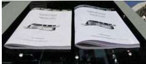
Booklets with ISG (cold glue) left and conventional stitching (right)
