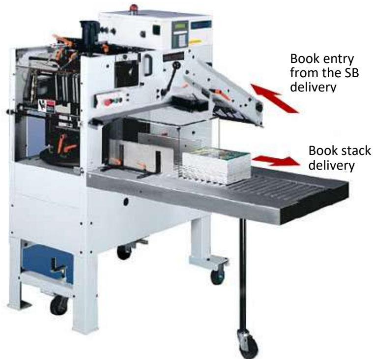
Book stacker BSS-10: for in-line connection to the Smart-binder delivery conveyor
