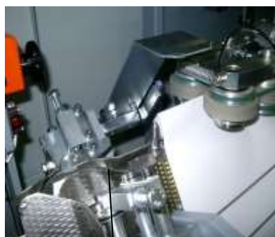
ISG Cold-Glue Application Nozzle on the Smart-binder
