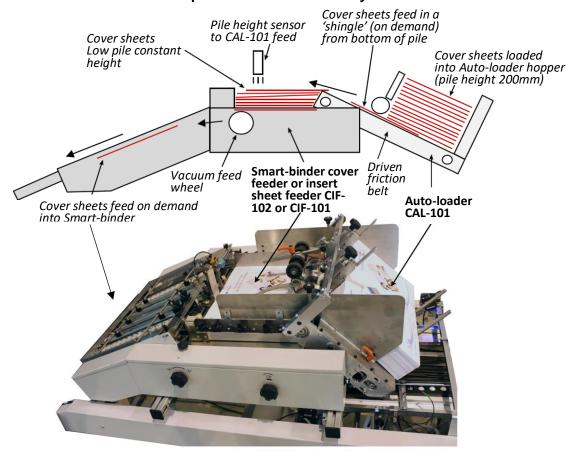
The operator may load a large quantity of covers (up to 200mm pile height) into the CAL-101 Auto-loader. The covers feed out automatically from the bottom of the Auto-loader in a 'shingled' stream.
