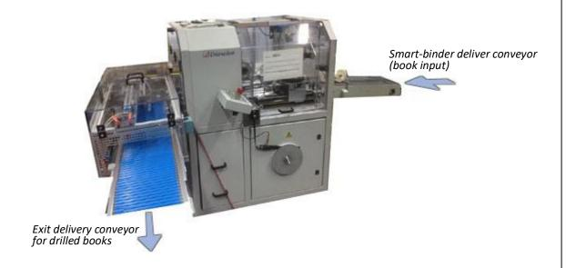
The advantage of the HDM-100 over the optional hole punching module <u>CHP-100</u> is that the HDM-100 can insert holes in books **up to the Smart-binder maximum of 10mm thickness**.
