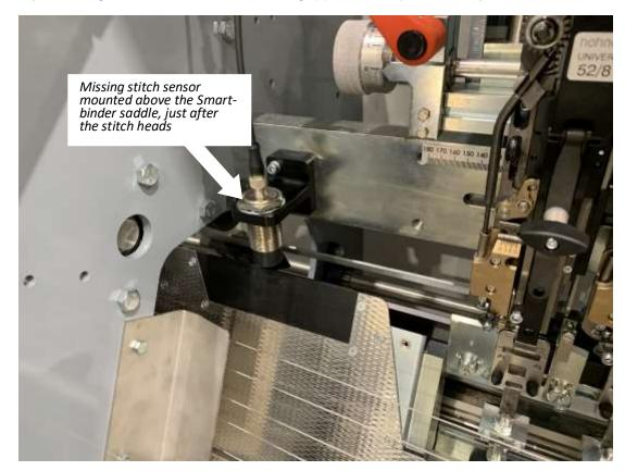
If a staple is detected as being missing then the Smart-binder will reject this booklet. The machine will stop automatically, and display a message on the touch screen, if there are a 3 or 4 consecutive rejected booklets with missing staples.
