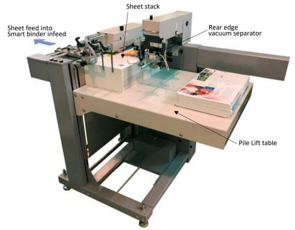
The feeder may be loaded with piles of pre-collated sheets. An optional loading trolley options PLT-100 (or HPL-100) are available to assist loading The maximum pile height is approx 700mm (27.56") but actual pile heights depends on a number of factors (the top sheet must remain relatively flat).
