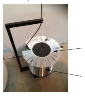
Wire spool holder with brush to resist wire unwinding.
