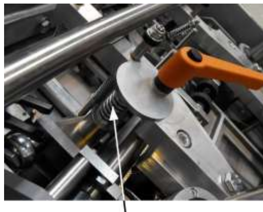
Hole punch installed in trimmer
