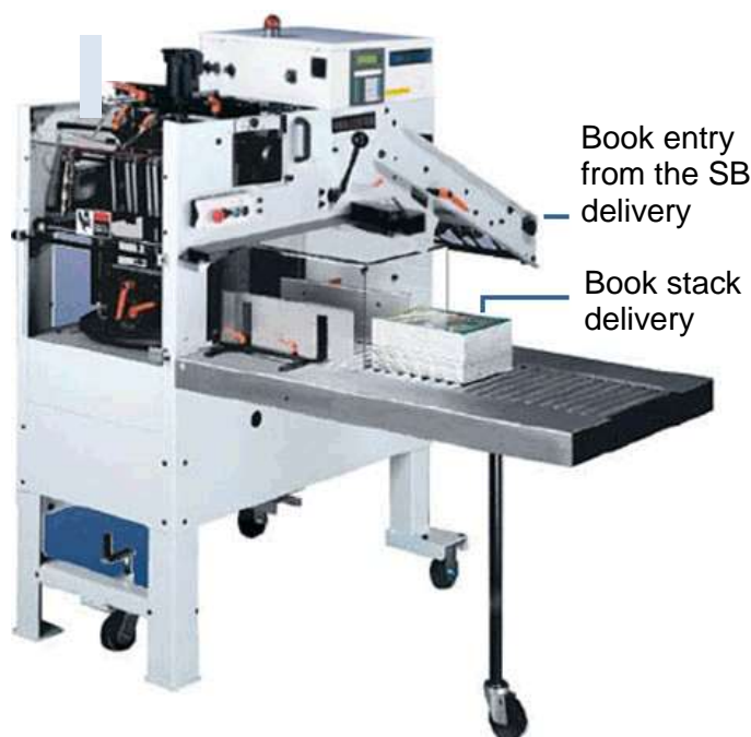
The BSS-10 book stacker: for in-line connection to the Smart-binder delivery conveyor
