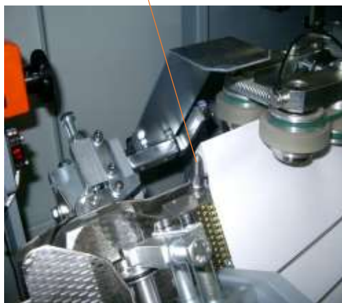
ISG Cold-Glue Application Nozzle on the Smart-binder
