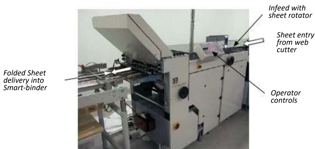
RF-100 rotator/folder unit positioned before the SB infeed
